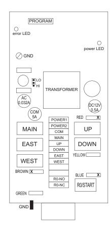
Fig. 1 Internal Layout Diagram
